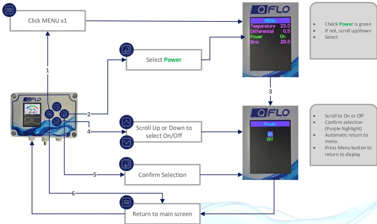
**Figure 2: Power ON/OFF Process**
