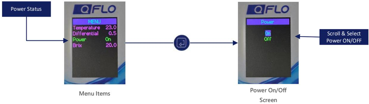
**Figure 1: Power ON/OFF Displays**
